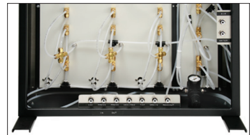
Rear of panel showing quick-connect hookups and plumbing.
