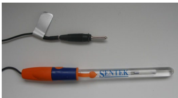
Figure 30 : Calomel (HgCl) Reference Electrode
