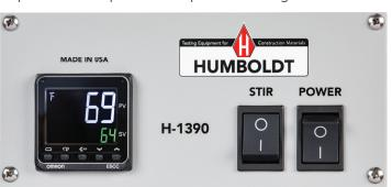
Humboldt Water Baths are fully insulated to help maintain constant temperatures easily. Models H-1390 and H-1392 can accommodate (12) 4" diameter or (3) 6" diameter Marshall specimens at a time. And the model H-1394
