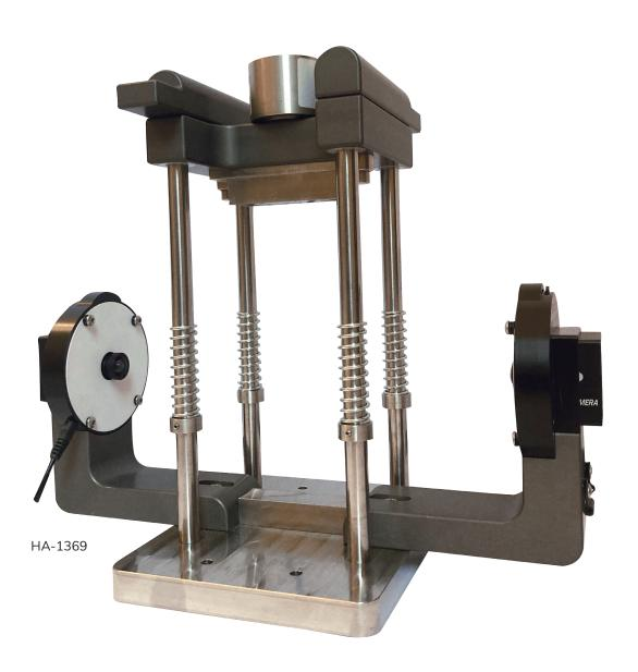
MiAS is an advanced image analysis system designed specifically to enhance monotonic BMD (Bulk Material Density) tests. Leveraging the power of Digital Image Correlation (DIC), MiAS offers an innovative solution for testing materials by integrating cameras, artificial intelligence (AI), and consistent illumination. MiAS improves upon traditional testing systems such as I-FIT, Ideal CT, and IDEAL RT frames by offering a more accessible, cost-effective, and efficient solution.
