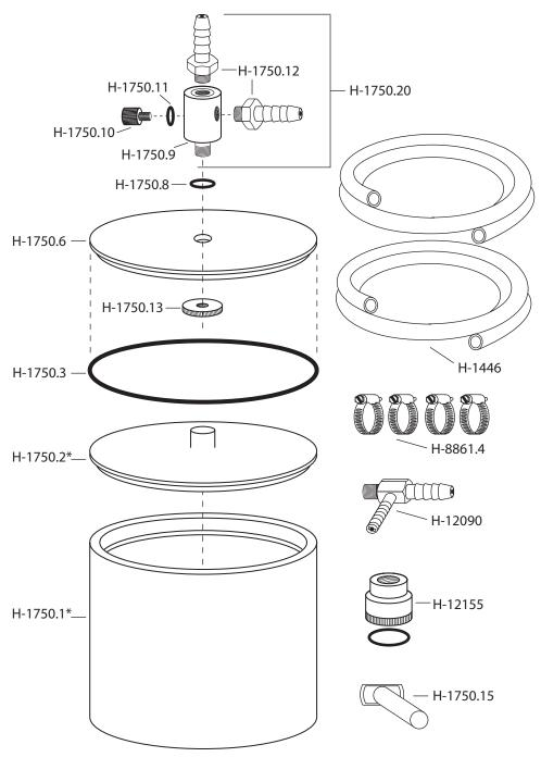
\*For Stainless Steel Model, H-1750SS, substitute H-1750SS.1 and H-1750SS.2 \* For H-1751, 1500g capacity model, substitute H-1751.1
