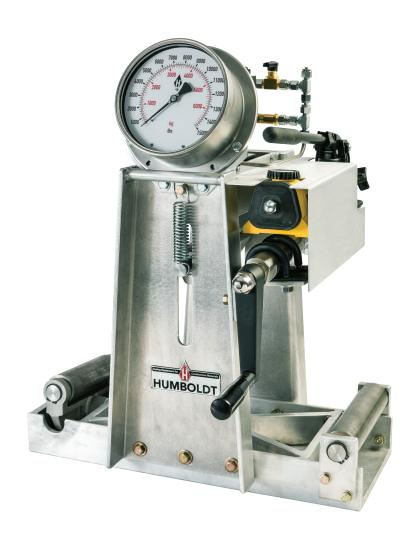
Continuous Load Concrete Beam Testers
