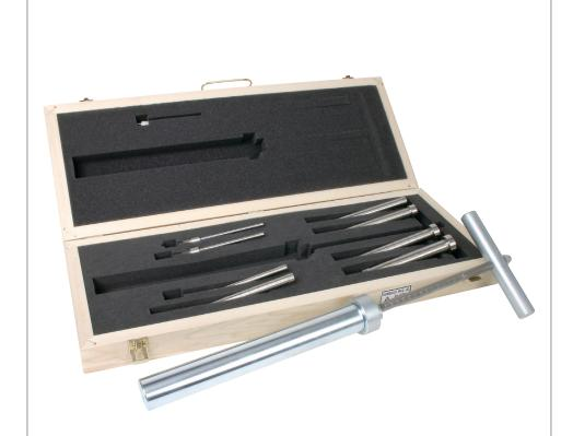
Mortar Penetration Resistance Apparatus
