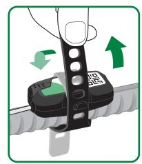
Pull strap tight over the installation hook and fold remaining strap over
