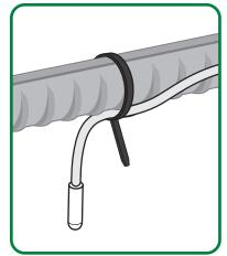
Secure the cable and temperature probe below the rebar
