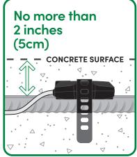
Install the transmitter on rebar no more than 2 inches (5cm) from concrete surface
