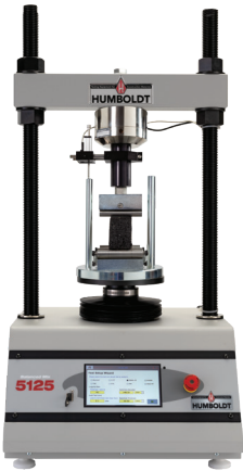
SCB (LSU Method) ASTM D8044
